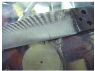
I carried out one of the quenching water and here is the result, the blade did not support. A slit on all bevel with cm of the beginning of the edge.
