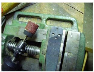
The heel edges are rounded with Dremel (sandpapering drum coarse grits.)
