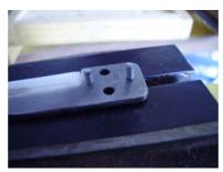
In order to carry out insertion in force of the tangs, protect the blade by applying a little electrician Scotch tape to bite of a small vice which you just sufficiently half-open in order to let pass the steel stems.
