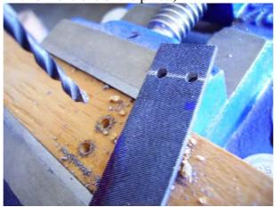
The two openings of the pivots are bored. One sees the line traced in order to have the two perfectly aligned holes.
