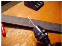
Once the latch finished, Carry out T with a nail stainless of 2,5mm, cut the head man (by wedging it in vices), using the discs to cut up Dremel. Then assemble the nail in the Dremel (or a drilling machine) chuck and apply the two seconds at low speed to a file in order to decrease very slightly the thickness in order to be able to insert without forcing the first mm in the latch. (Even process that for the tang pins).
