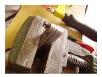
Put the pivot in the four handle part maintained in the vice and round with the drum of sandpapering coarse grits with 20000-30000 turns that goes rather quickly (less than two mn) On can also do it with the sander fixed on the bench. It will be the part which one will make go and to come on the tape.
