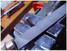
Then with the drum coarse grains of Dremel, round each end of the latch by taking care not to remove too many matter and kill thus the hole.
