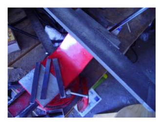
The 4 pieces of the handle are cut, now it is necessary to rectify the irregularities and, if it is not the case, to put all the handle at the same width. (Some files inevitably do not have the same width on all length.) To put them the same width, I use the enormous file at side, it is hyper abrasive and effective. If not for the lazy ones or people equipped, the right angle driver or the sander coarse grains will make the deal very well.
