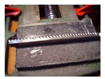
Attack with  $45^{\circ}$  in direction of the pivots of the handle (moreover it is a compromise between toxification and "guillochage").
