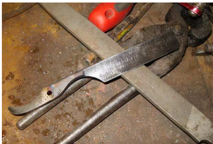
After the quench, the sharpening file slide on the edge.
