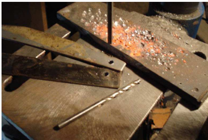
I drilled to 3,8mm, reamed to 4mm, and drilled the heel to 4mm
