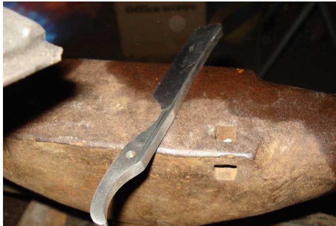
I chequered the back, 3 normalization, oil hardening.
