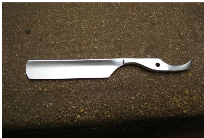
I countersunk the side of the blade, and clean it with a 500 grit belt. I'm between, 0,09 and 0,13 mm
