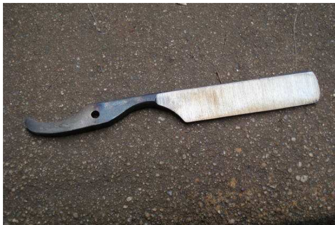
After the quench, the sharpening file slide on the edge.
